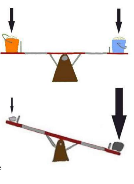
"We make the heavier side have a smaller force by moving the heavier object closer to the middle and the lighter side have a bigger force by
